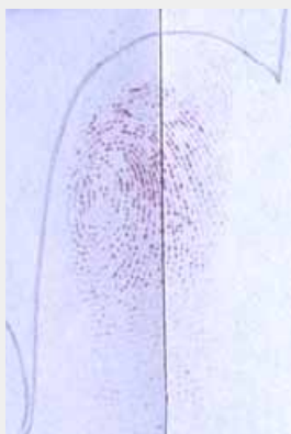
Fingerprint cut in half then treated: 5-MTN (left) compared to ninhydrin (right) in daylight (BVDA International).
