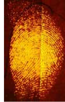
Fluorescence of DFO (left) vs 1,2-IND (right) with green light & dark orange filter (BVDA International).
