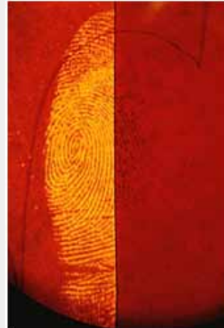
Fluorescence of 5-MTN (left) after treat- ment with zinc chloride (green light & dark orange filter) (BVDA International).
