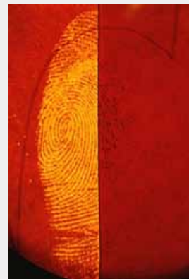
Fluorescence of 5-MTN (left) after treat- ment with zinc chloride (green light & dark orange filter) (BVDA International).
