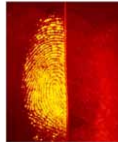
Fluorescence of DFO (left) vs ninhy- drin (right) with green light & red filter (BVDA International).
