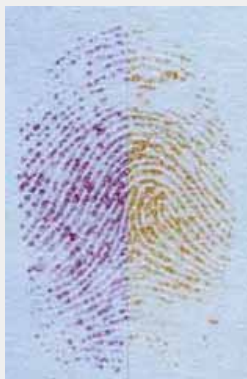
Treated with zinc chloride following ninhydrin (right)
