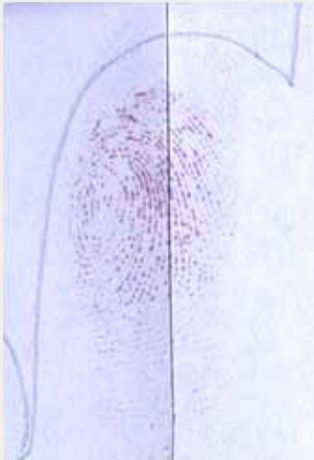
Fingerprint cut in half then treated: 5-MTN (left) compared to ninhydrin (right) in daylight (BVDA International).
